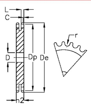
C = 2 D = 25 De = 305.7 Dp = 298.27 For chain size =  $5/8 \times 3/8$ For chain type = 10 B-2 h2 = 25.5
